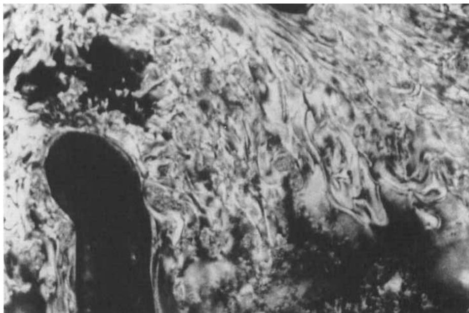
FIG. 7. Polarized light micrograph of a polymerized LCT mixture.
